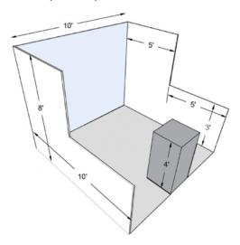
Linear booths consist of an 8' high back drape and 3' high side dividers mounted on aluminum tubular frames. Perimeter booths may rise up to 12'. Solid construction more than 4' high must be a minimum of 5' back from the aisle.
