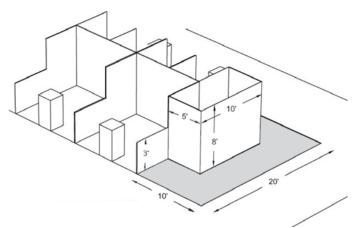
An end-cap booth is exposed to aisles on three sides and composed of two booths, generally 10' deep by 20' wide. The back wall must not exceed 8' in height and only the rear half of the booth space. The back wall is restricted to 4' high within 5' of each aisle, permitting adequate line of sight for the adjoining booths.
